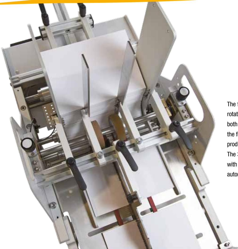
The feed selection uses rubber counter-rotating rollers with micro adjustments on both the left and right side, which make the feeder extremely flexible for any type of product.
