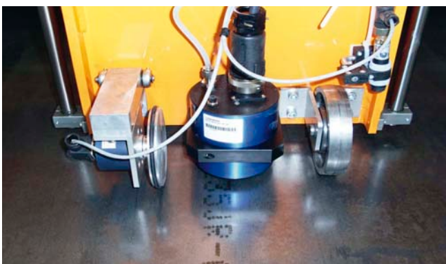
Steel sheet marking with etching ink
