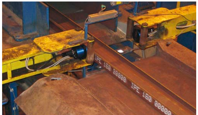
Marking of H-beams
