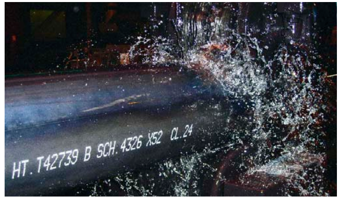
Steel tube marking with pigmented MEK ink
