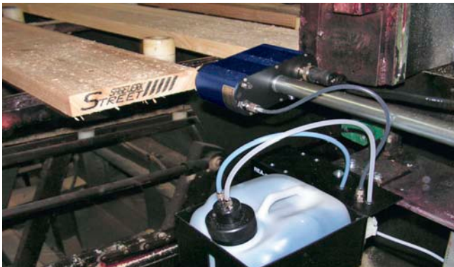
Marking on rough sawn timber boards
