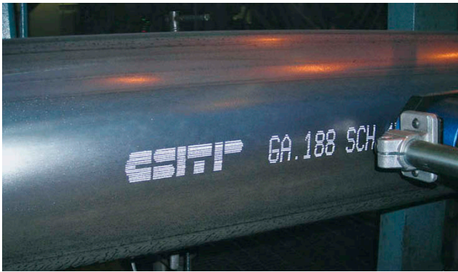
Marking of steel pipes
