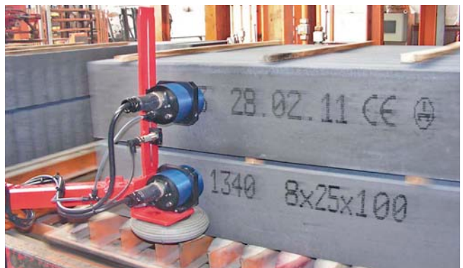
Coding of precast concrete elements
