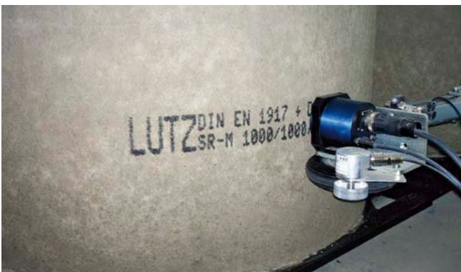
Marking of precast concrete pipes
