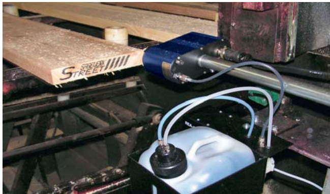
Marking on rough sawn timber boards
