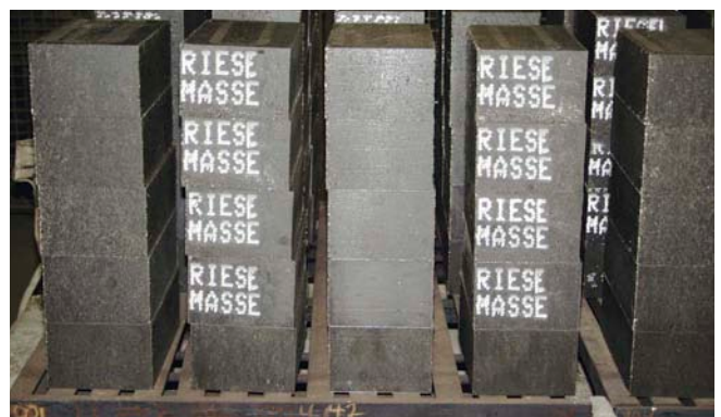
Refractory stone marking with high-temperature ink
