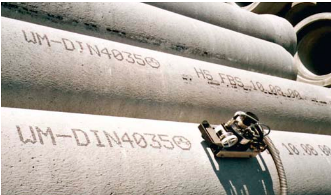
Mobile marking of concrete pipes
