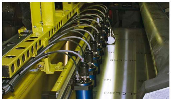
Coding of oiled metal sheets with acetone ink
