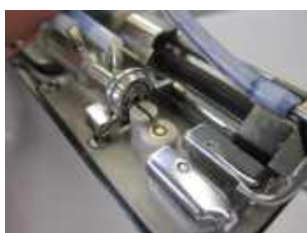
Mount the new drop production body back on the adapter of the ground plate.
