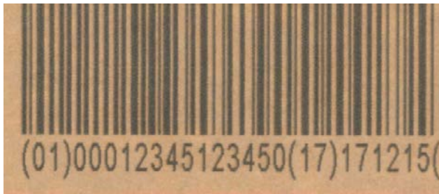
European GS1-128 barcode printed with an industry leading at 6 mm print throw distance. Industry-leading ink throw distance provides consistently higher quality print despite the irregularities of factory floor environments.
